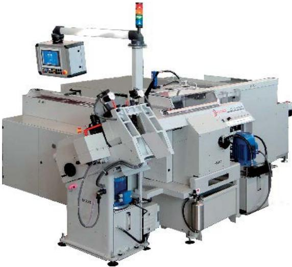
The ATLAS-1120 Dual combines automatic strip cutting with the push-through counter-pressure punching process and is therefore an important high-performance production line for the finishing of labels punched in stacks, as well as for "scratch" and "loyalty" cards.
